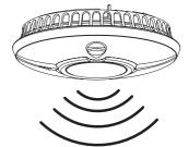
**NOTE:** The button tests the alarm's smoke sensing circuit. There is no need to test your alarm with smoke. If your smoke alarm fails to give an audible test signal, please refer immediately to Troubleshooting, at the end of this manual.
