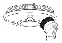
Your smoke alarm may false alarm when it is being cleaned using a vacuum cleaner.
