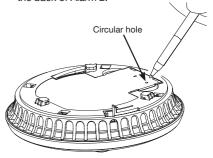
The red LED next to the learn button will flash briefly then light up for approximately five seconds to show that it is ready to receive the "learn in" signal. During these five seconds you will need to briefly press the test button on Alarm 1 to wirelessly interlink the two alarms.
