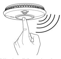
b Your alarm will silence and enter into a reduced sensitivity reset cycle for approximately 10 minutes.
