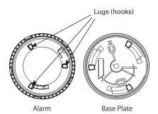
When used with the base plate, the alarm can be attached in any orientation, simply line up the lugs (hooks) with the holes at the end of the slots then twist the alarm clockwise until the alarm stops, make sure the alarm is twisted on fully.
