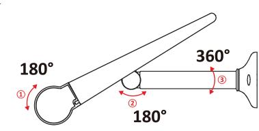
(1) Rotate the lamp head to adjust lighting directions, 180° adjustable.
