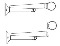
The lamp head can be removed according to the arrows on the side of the lamp for split installation.
