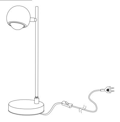
**Note:** This light is designed with adjustable height, press the pin on the canopy to adjust the height of the light.
