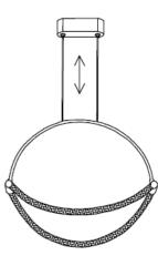
The height of the luminaire is adjusted by the tensile head.
